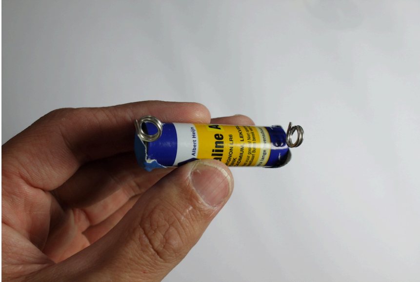
Fig. 1 - The battery with coils attached to make a magnet
